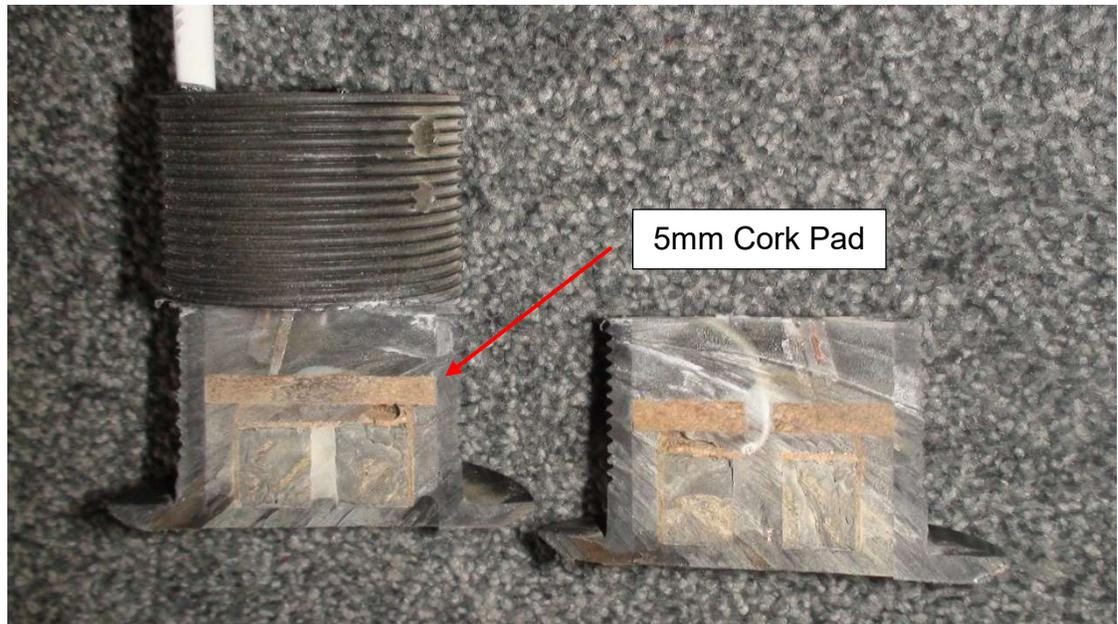
Figure 11 - Cross sections of CruzPro ATU120BT
