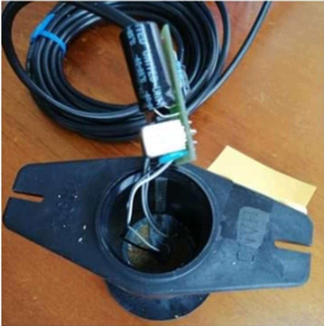
*Figure 13 - ATU120BT depth sounder. PCB Before potting*
