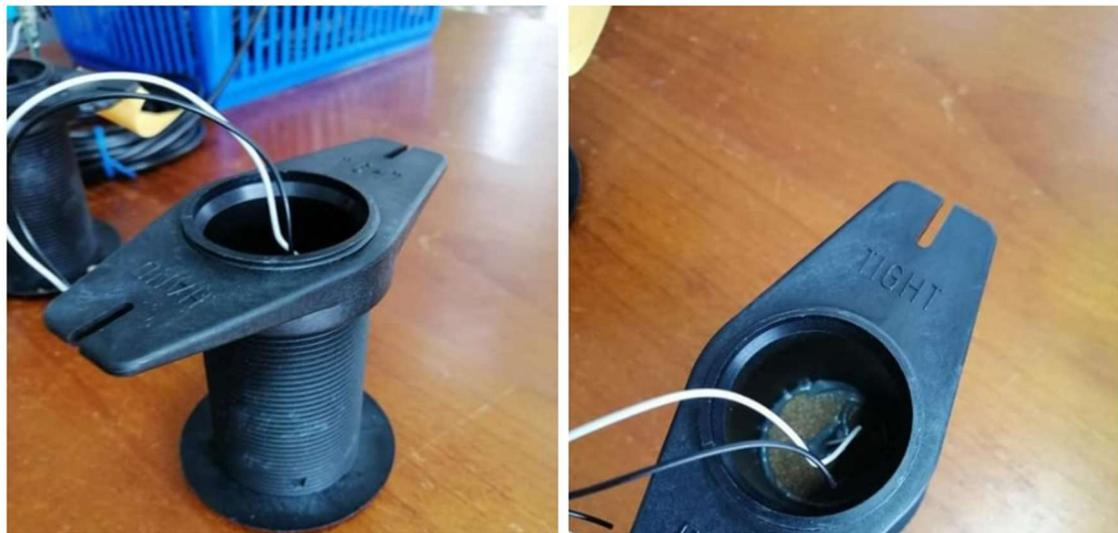
Figure 12 - ATU120BT depth sounder. Before potting electronics
