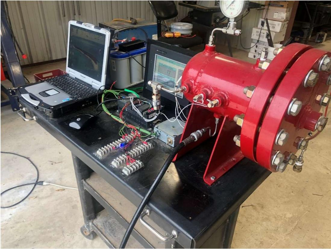
*Figure 2 Test Chamber with transducer installed*
