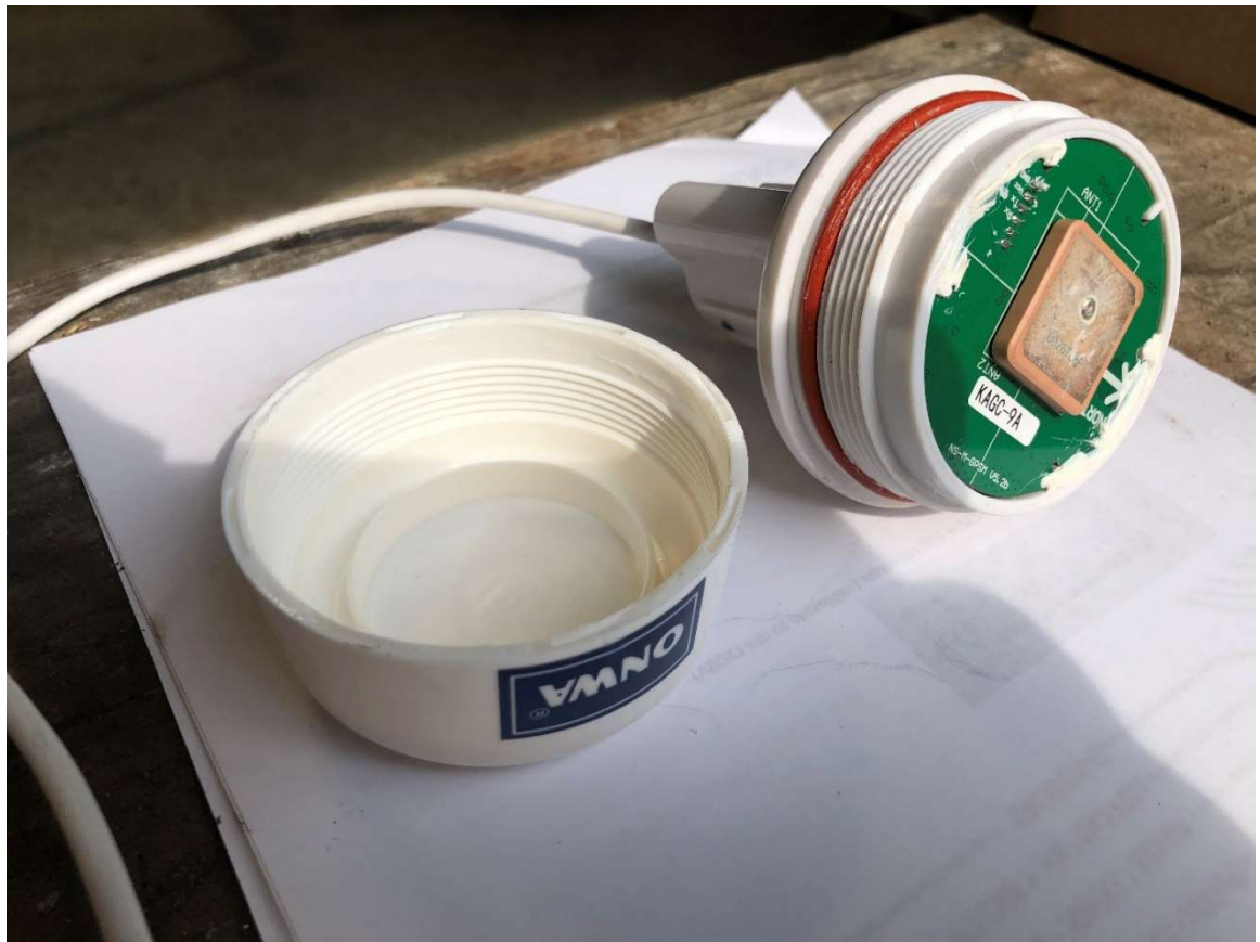
Figure 7 – Units opened up to show PCB
