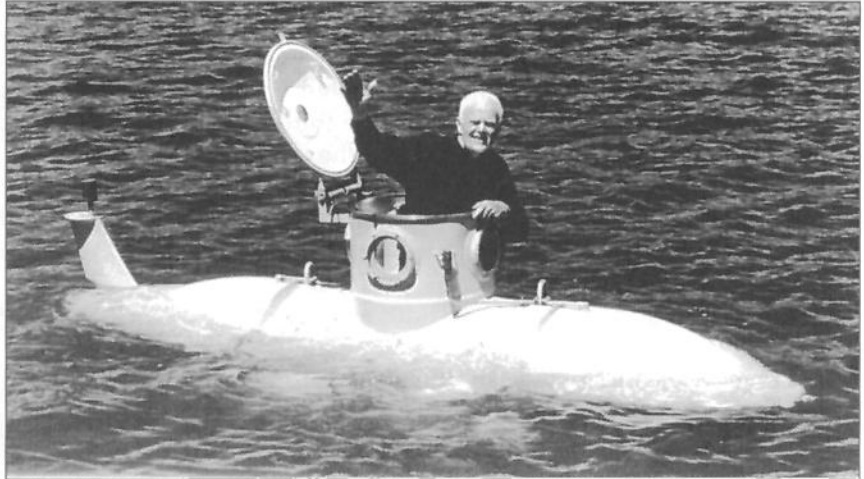
K-350 submarine. Note the sonar transducer on the raised fin.
