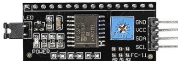
Typical I2C backpack for LCD
