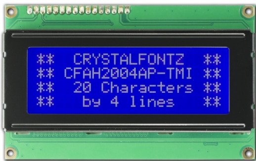
Typical 20x4 LCD Character Display
