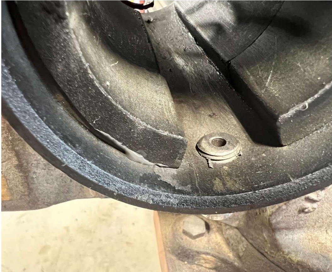
Figure 29 – Swagelok Fitting, Part #: SS-400-1-4 before machining flush
